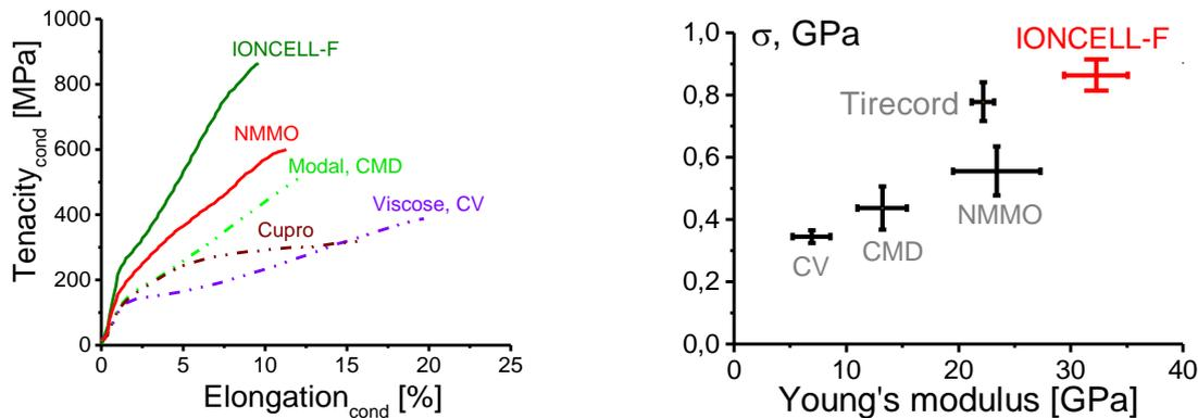
Figure 2, Left: Stress-strain curve of the Ioncell-fiber and of commercial regenerated cellulose fibers. Right: tensile strength vs. Young's modulus of Ioncell fiber in comparison to commercial regenerated cellulose fibers.
